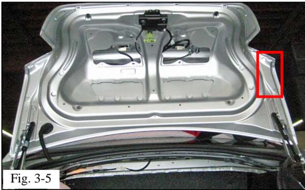
(j) Beginning with the RHS underside installation template, locate the general installation area on the inner sheet metal of the trunk lid (Fig. 3-5).
