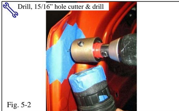
(c) With the 15/16" hole saw, insert the hole saw pilot drill into the previously drilled 3.0mm pilot hole. Carefully drill until the hole saw has cut the 15/16" hole (Fig. 5-2). Use the shop vacuum to collect the shavings when drilling the holes.
